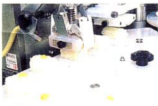
Shari dama are shaped as if by hand through a patented two-stroke action.
