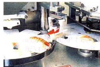
The sushi is transferred to the wrapping section of the system, where each piece is individually wrapped.
