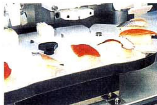
On the turntable, wasabi is automatically applied and the topping is added (topping operation is manual).
